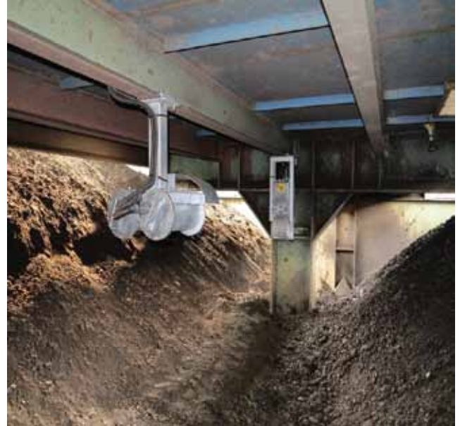
Mine dust monitoring system. Detector and radiation emitter (ATEX version)
