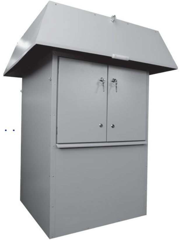
PI-MSKA 02 POW meter for measuring radioactivity air - general view.
