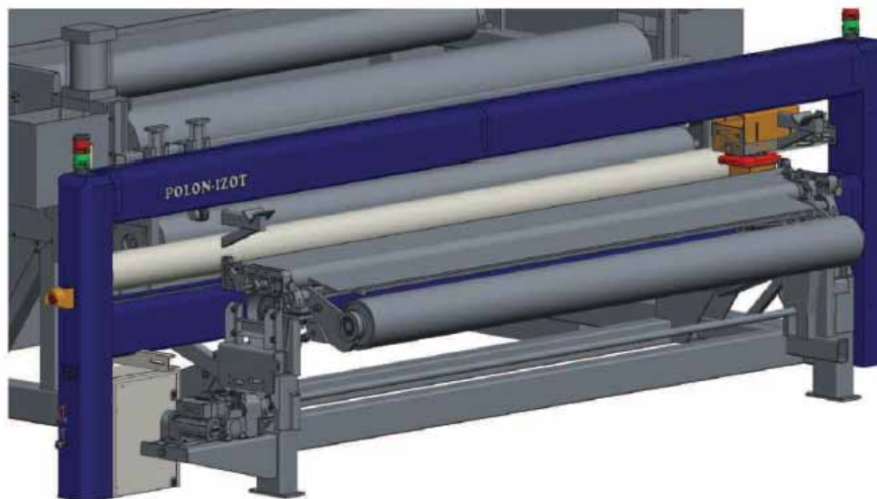
Example: on-line basis weight gauge integrated in the production line
