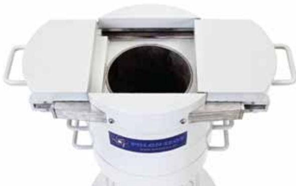
View of an empty, open measuring chamber.
