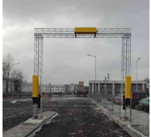
PI-MSKA system with a top detector and two detectors placed opposite each other
